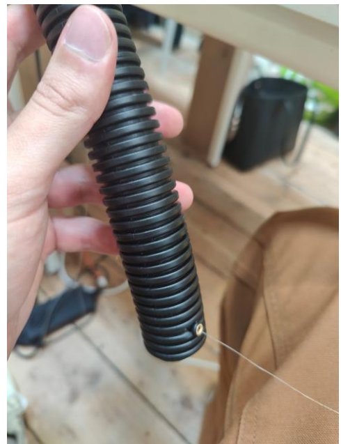
How the wire is supposed to exit the stem and be pulled by the servo. Made a cool solution with the hole so the tension and stress will be less on the wire.
