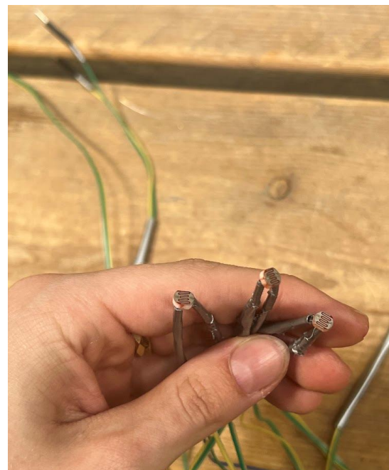
LDR sensors have been soldered
