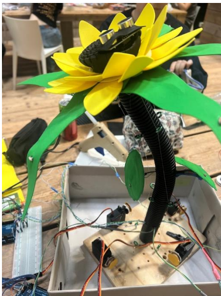
Wiring and attached a piece of foam to hide the Ultrasonic sensor a bit more for aesthetics
