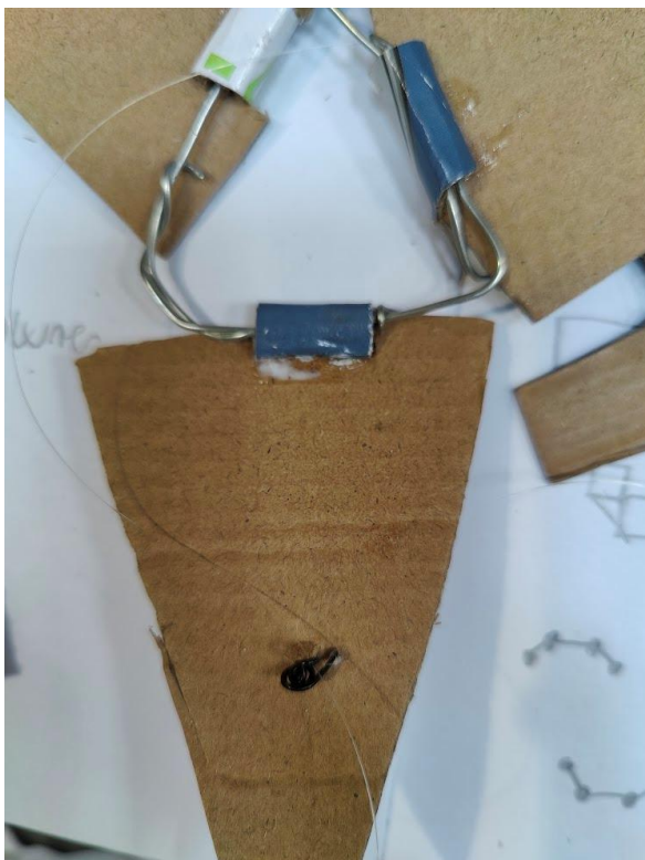
Metalwire frame for the cardboard to be able to flip up and down
