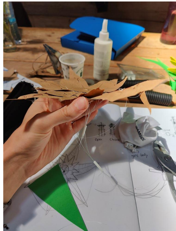
A retract and pullback mechanism split in two. One pulls and closes the leaves, one pulls and opens the leaves
