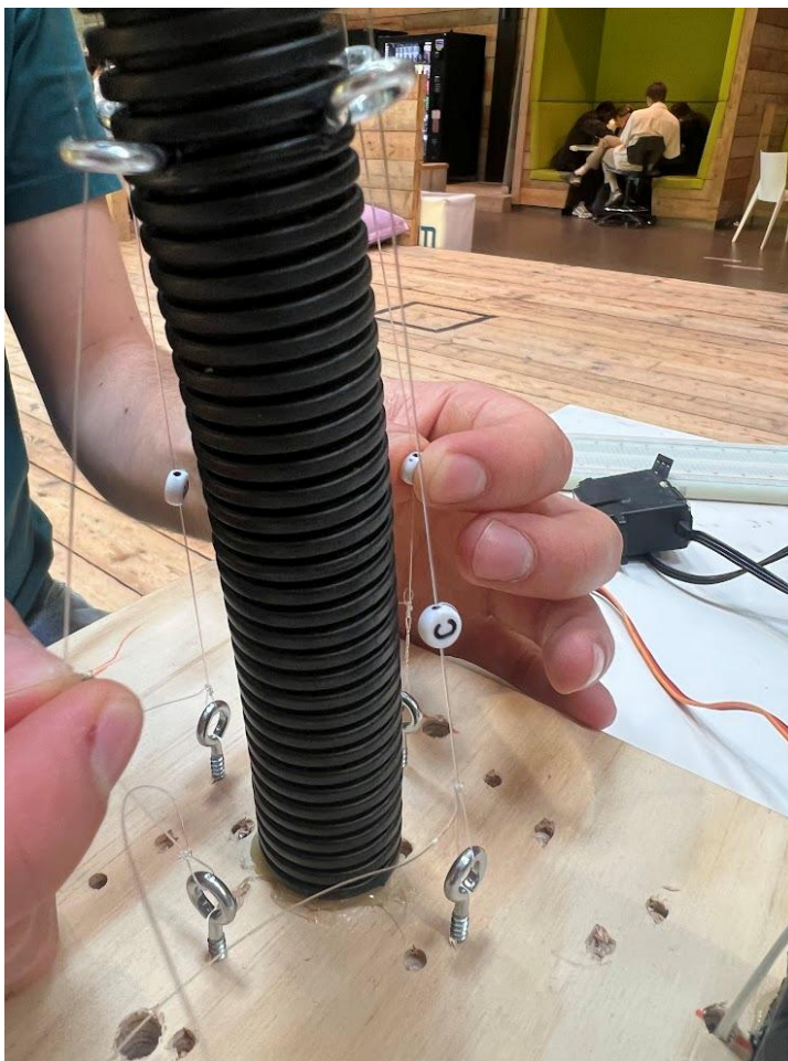
Honorable mentions by my fellow groupmembers. Really functions well with the weighted string to make the servo contra pull, which makes it easier for it as well
